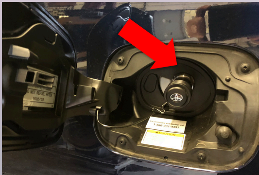
Fuel Fill Receptacle Cover in Place
