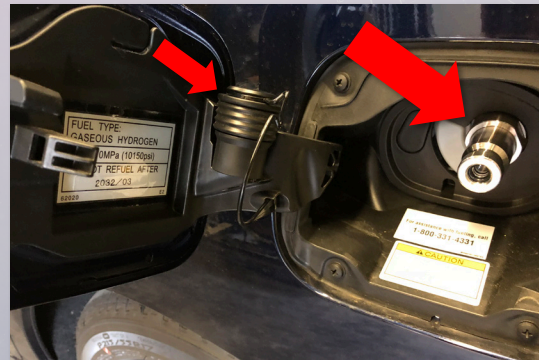
Fuel Fill Receptacle Cover Removed
