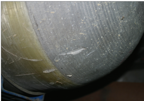
Scuffing Damage on Type 2 Cylinder
