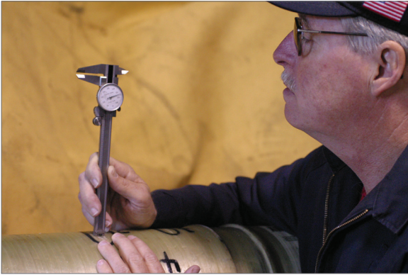
Measuring Depth with Veneer Calipers
