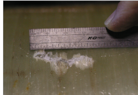
Surface Cut Under 1 Inch
