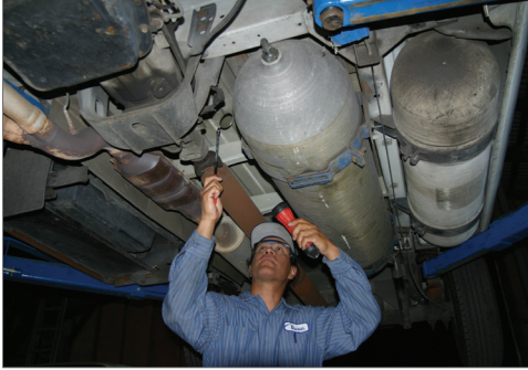
You Must Be Able to Inspect All 360° of the Cylinder Surface
