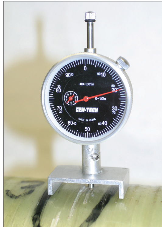
Measuring Depth with Dial Gauge
