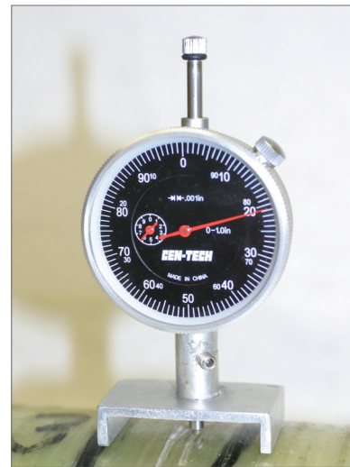
Measuring Depth with Dial Gauge
