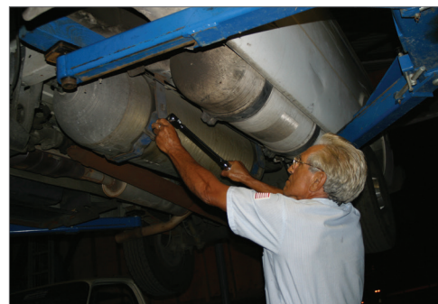
Check Torque on Mounting Brackets
