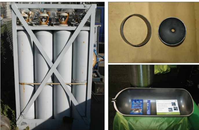
Cascade of Type 1 all Steel Cylinders
