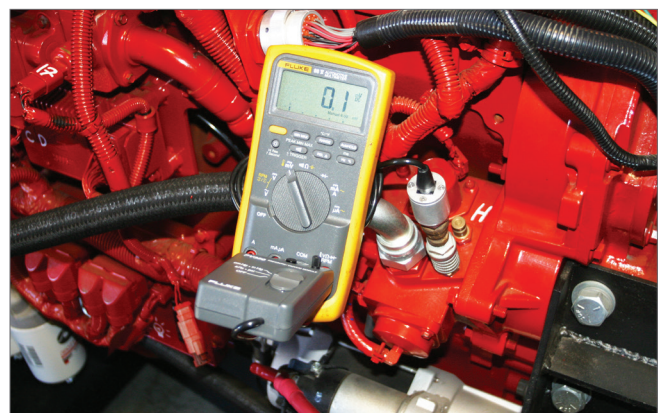
Checking Secondary Pressure with Electronic Gauge
