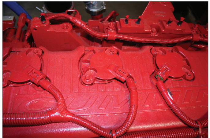
Separate Coils for Each Cylinder
